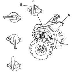
NOTE: Return the valve to the ON position after refueling.
